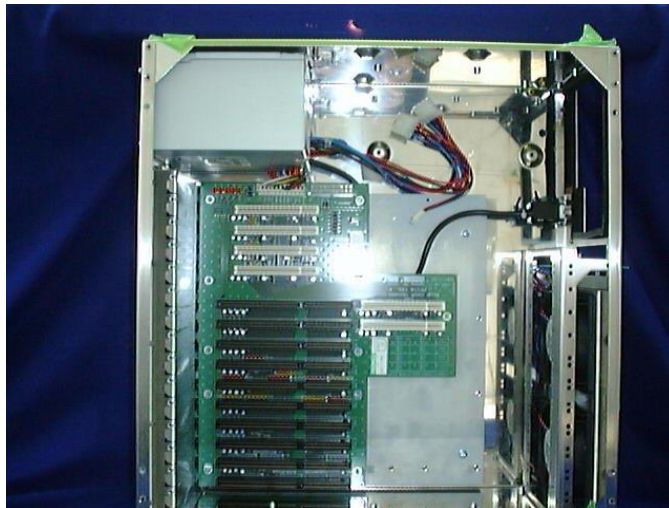
PSU sub-assembly in Chassis
