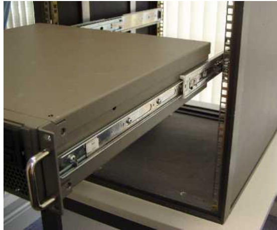
Figure 24: Insert Chassis into Cabinet
