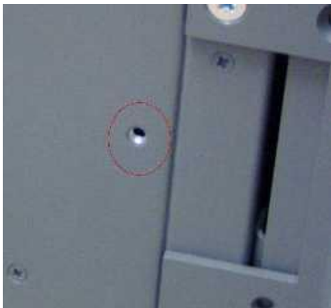
Figure 17: 4U front mounting hole
