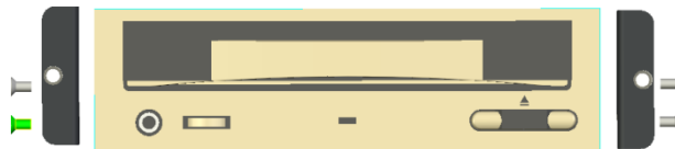
Figure 10: 5¼ device mounting ears and screws
