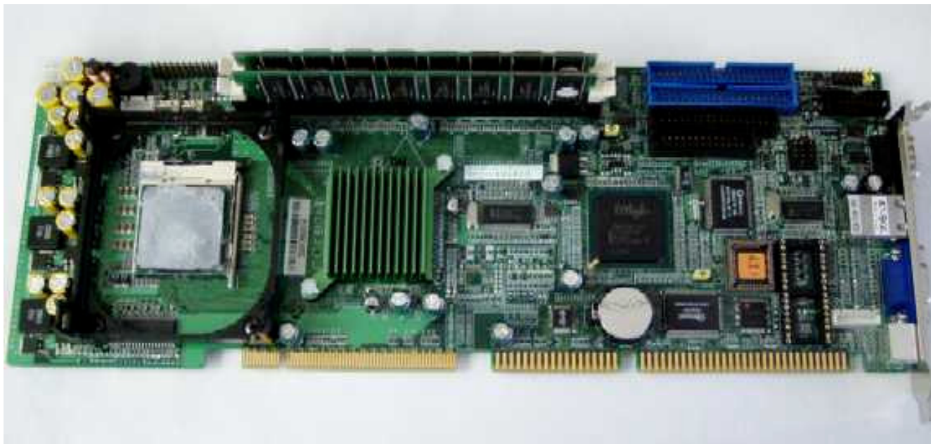
Fig 1: Full-length BCT-PICMG-P4 Single Board PC
